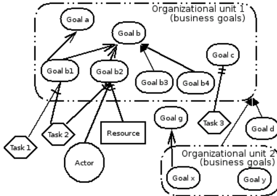
Fig. 1. The concepts of the i^* model adapted to support ISO/IEC 15504 process models
